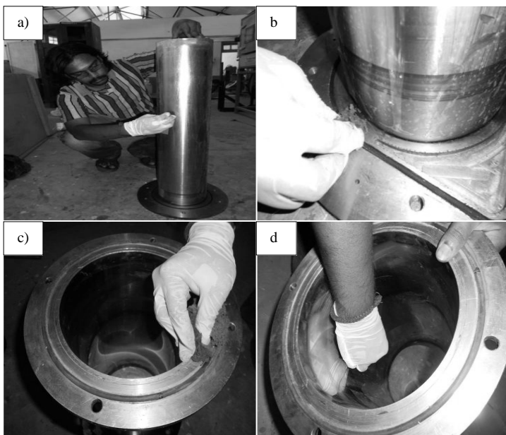
Fig. 6. Rubber O-ring fitted within the groove
