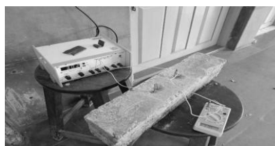
Fig. 3. Experimental set-up for measurement of electrical resistivity
